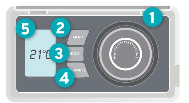
Press down the **dial**, and the display screen shows you the thermostat target temperature and timer mode.
