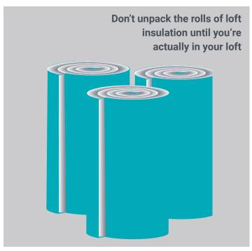
Most insulation is compression packed and will expand once the wrapping is removed, so only unpack the rolls once they're up in the loft. It's also much easier to cut the insulation while it's still rolled up. You may find that the packaging has a perforated line indicating the required width to the cut the insulation so that it fits neatly between the joists. Often the rolls will be pre-cut to the correct width before they are packaged.
