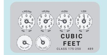
The first dial shows the pointer right above the number 7. Now look at the second dial. This is 1, so it means that the dial before has passed the 7. The full reading for this dial meter is **7120**.
